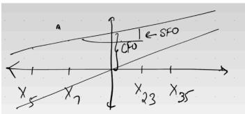
Even after initial CFO correction, some small errors (residual CFO) and sampling frequency offsets (SFO) can still remain, leading to further phase distortions over time.
