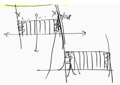
Guard bands are portions of the frequency spectrum at the edges of the OFDM signal that are left unused to prevent interference with neighboring signals or systems.
